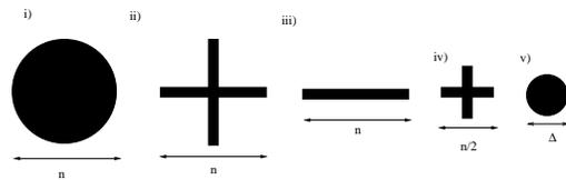
Fig. 2. Prototypical generic shapes used in the ballistic deposition computer experiment. The diameter  $\Delta$  in the last shape of this figure is defined by the constrained area of the circle which should match  $n$  pixels, i.e.  $\Delta = 2\sqrt{n/\pi}$
