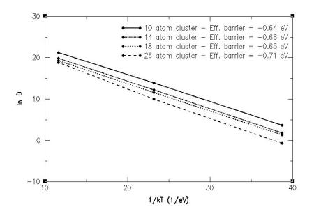
Figure 7. Arrhenius plot with the effective barriers for the 10 atom, 14 atom, 18 atom and 26 atom clusters
