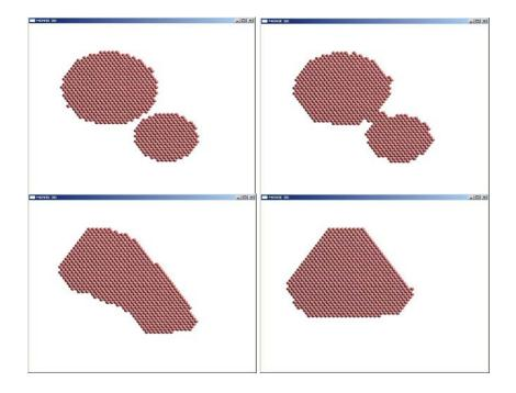
Fig. 8 Results of KMC simulation of the coalescence of two islands performed at 400K
