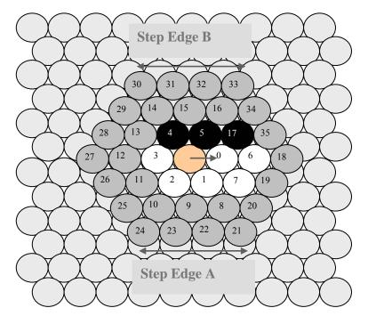
Fig. 4. Three shells of nearest neighbor atoms around the central atom (atom selected to move) and the pattern recognition scheme.
