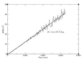
Fig. 6 Mean square displacement of the CM for a 100 atoms at 500K
