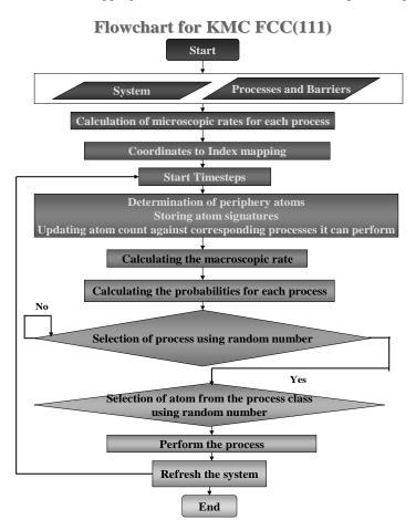
Figure 3. Flowchart for a kinetic Monte Carlo simulation
