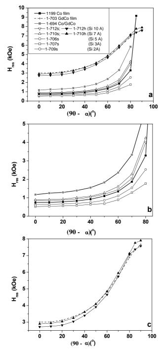
Figure 17. Dependence of the resonance field of  $\{Co(70 \text{ Å})/Si/(Gd-Co)(120 \text{ Å}))/Si\}_4/Co(70 \text{ Å})$  multilayers on the thickness of Si sublayer for  $\alpha = 90^\circ$ , f = 10.45 GHz.
