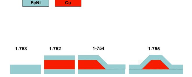
Figure 1. Ni<sub>80</sub>Fe<sub>20</sub> based thin film structures studied by FMR.
