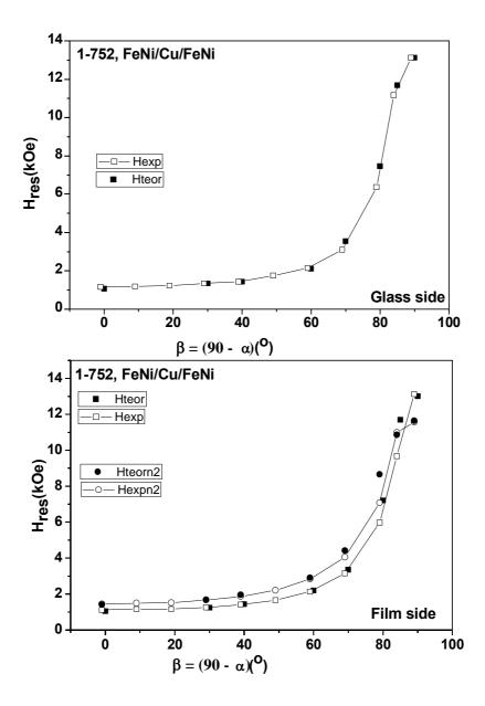
Figure 12. Theoretical and experimental angular dependencies of the resonance field of  $Ni_{80}Fe_{20}$  /Cu/  $Ni_{80}Fe_{20}$  part of multilayer deposited with opening the vacuum chamber, f = 10.45 GHz, room temperature.
