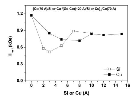
Figure 20. Influence of the thickness of non-magnetic sublayer on the width of FMR line of  $Co(70 \text{ Å})/Cu/(Gd-Co)(120 \text{ Å}))/Cu}_4/Co(70 \text{ Å})$  multilayers
