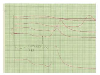
Figure 22. FMR signals for sample 1-720 ("zero" field signal is present).
