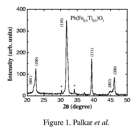
**Figure 1** X-ray diffraction pattern of  $Pb(Fe_{0.5}Ti_{0.5})O_3$  sample. Lines marked with '\*' are from  $Pb_2Ti_2O_6$  impurity phase.
