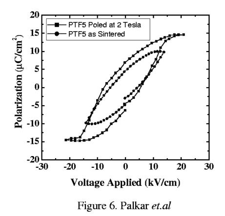
Figure 6. Ferroelectric Hysteresis Loop of Pb(Fe<sub>0.5</sub>Ti<sub>0.5</sub>)O<sub>3</sub> pellet sample, a) as sintered,
