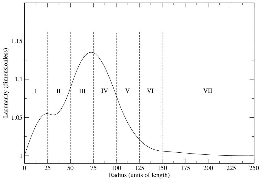
**Figure 10:** The analytically calculated self-referred lacunarity curve for a cross with dimensions  $L_1$  and  $L_2$  of 100 and 50 units of length respectively.
