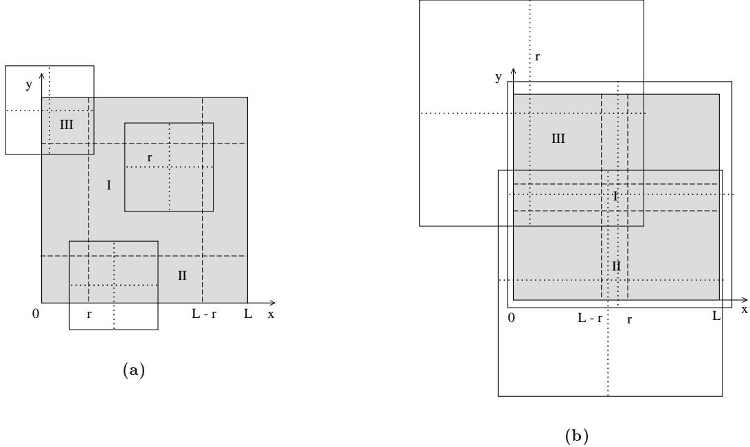
**Figure 1:** Square regions that correspond to the self-referred lacunarity calculation for the intervals (a)  $r \in [0; L=2]$  and (b)  $r \in [L=2; L]$ . The sliding windows in the region I are completely filled in (a) and capture all the square in (b). In the regions II and III they are partially filled in (a) as well as in (b).
