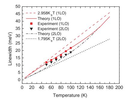
FIG. 2: Linewidth of sidebands with one and two phonons as functions of temperature. The lines are the calculated results, and the filled symbols are the measured data.
