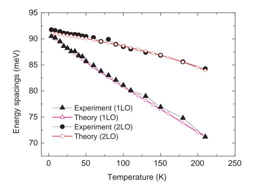
FIG. 3: Temperature dependence of the energy spacing from the sidebands with one and two phonons to the zero-phonon line obtained from the theory and from the experiment.
