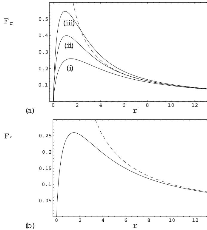
Figure 1.3. The force near the dislocation line: (a)  $F_r$  and (b)  $F_t$ , with  $\nu = \frac{1}{4}$ ;  $\frac{5}{4}$  are given in units of  $b_x b_x^0 = 2(1 - \nu)$ . The dashed curves represent the classical force components.
