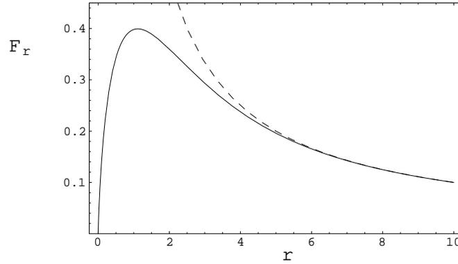
Figure 1.1. The Peach-Koehler force between screw dislocations is given in units of  $b_z b_z^0 = [2]$ . Nonlocal elasticity (solid) and classical elasticity (dashed).
