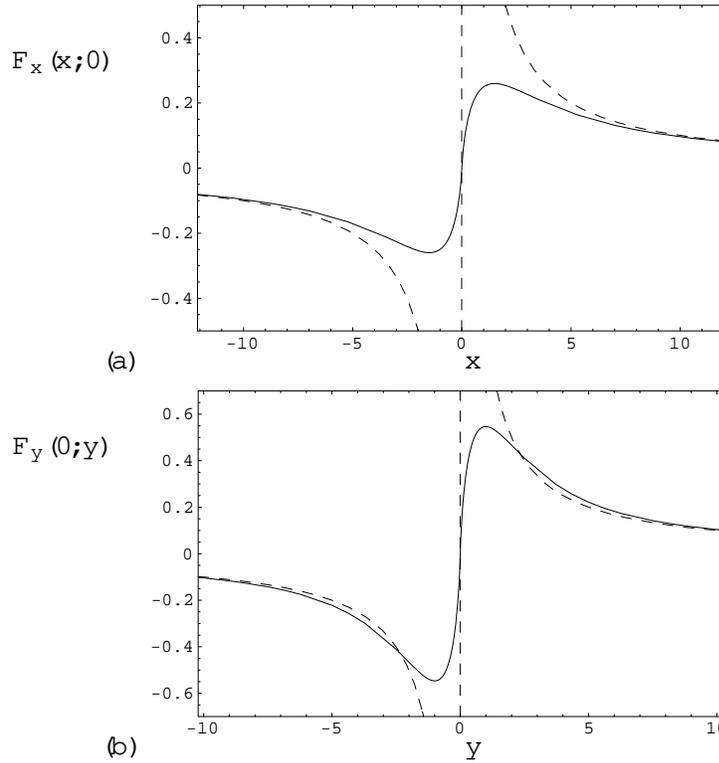
Figure 1.2. The glide and climb force components near the dislocation line: (a)  $F_x(x;0)$  and (b)  $F_y(0;y)$  are given in units of  $b_x b_x^0 = [2(1 - \nu)]$ . The dashed curves represent the classical force components.
