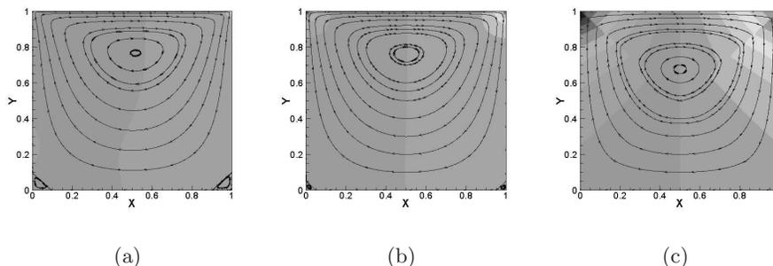
FIGURE 3. Density isocontours for (a)  $\text{Kn} = 0.001$ , (b)  $\text{Kn} = 0.01$ , and (c)  $\text{Kn} = 0.1$  (the variation of the density is  $0.995 \leq \rho \leq 1.005$ ). Superimposed are the streamlines.
