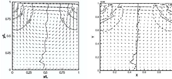
FIGURE 2. Flow in a micro-cavity for  $\text{Kn} = 0.1$  and  $\text{Ma} = 0.14$ : DSMC simulation (Jiang *et al.* 2003) (left) , velocity vector plot and density isolines from ELBM (solid lines) with the DSMC density isolines (dashed lines) superimposed (right).
