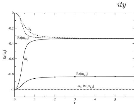
FIGURE 1. Real part of the solutions of the dispersion relation (equation (3.9)). Roots  $\omega_{2,3}$  and  $\omega_1$  correspond to Grad’s subsystem (equation (3.6)). The real-valued root  $\omega_6$  and the complex conjugate roots  $\omega_{2,3}$  are extended hydrodynamic modes.
