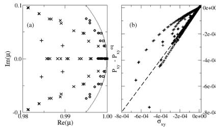
FIGURE 6. (a) Leading eigenvalues of the minimal kinetic model at steady state (square:  $\text{Kn}=10^{-4}$ , circle:  $\text{Kn}=10^{-3}$ , X:  $\text{Kn}=10^{-2}$ , +:  $\text{Kn}=10^{-1}$ ); (b) Scatter plot as in Fig. 4(a) for a state perturbed away from the steady state along the leading eigenvector ( $\text{Kn}=10^{-3}$ ).
