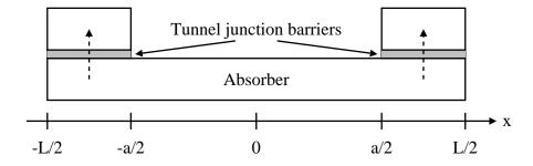
Figure 1. Schematic of the cross section of the proposed detector (not in scale). D ashed arrows on the two sides indicate the excess quasiparticle tunnelling
