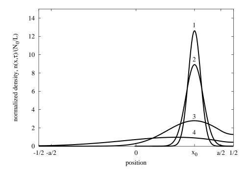
Figure 2. Temporal evolution of the density of excess quasiparticles in the device for an event occurring at  $x_0 = 0.3$ . Curves 1;2;3;4 correspond to  $= t_{loss} = 0.0005;0.001;0.01;0.5$ . The parameters used are =L = 1,  $t_{tunn} = t_{loss} = 143$ , a = 0.87
