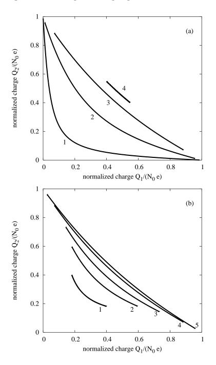
Figure 4. a) Collected charges  $Q_2$  vs  $Q_1$  for increasing values of =L;(0:25;0:5;1:0;5:0), tunn = loss = 143 and a = 0:871.b) Collected charges  $Q_2$  vs  $Q_1$  for increasing values of tunn = loss, (10:0;25:0;5:0:0;143:0;400:0), =L = 1,a = 0:871
