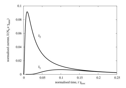
F igure 3. Tem poral evolution of the norm alised currents passing through the tunnel junctions for the absorption event located at  $x_0 = 0.3$ . Parameters correspond to =L = 1,  $t_{tunn} = t_{loss} = 143$ , a = 0.87
