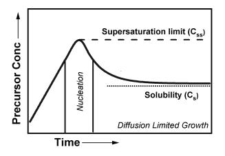
**Figure 4.** Reproduction of the generalized LaMer model plot describing nucleation and growth of crystallites versus time for continuous influx of precursor. Adapted from ref. 19.
