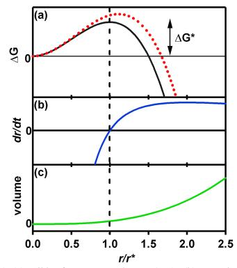
**Figure 5.** (color) (a) Gibbs free energy change ( $\Delta G$ ), (b) growth rate (dr/dt), and (c) crystallite volume plotted versus the crystallite radius, *r*, normalized by the critical radius, *r*\*. The activation barrier to nucleation,  $\Delta G^*$ , determined from the classical nucleation model (Equation 2) is indicated in (a). The dotted line in (a) (red) shows the reaction coordinate diagram for nucleation including destabilizing impurity ions.
