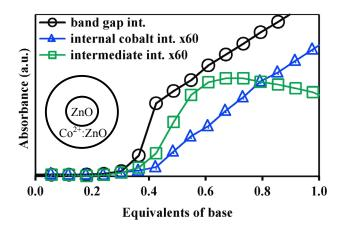
**Figure 3.** (color) ZnO bandgap ( $\circ$ ), intermediate Co<sup>2+</sup> ligand-field ( $\Box$ ), and Co<sup>2+</sup>:ZnO ligand-field ( $\Delta$ ) absorption intensities deconvoluted from the data in Fig. 1 by Single Value Decomposition, plotted versus added base equivalents (Adapted from ref. 18). The inset depicts the existence of undoped ZnO cores in the nanocrystalline Co<sup>2+</sup>:ZnO products.
