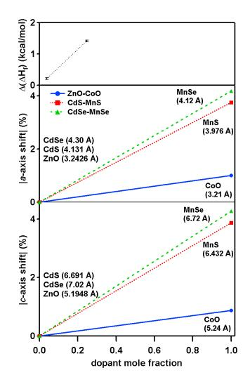
**Figure 6.** (color) (a) Enthalpy of formation of  $Zn_{1-x}Co_xO$  measured by dissolution in  $H_2SO_4(aq)$  plotted versus *x*, absolute values of the relative (b) *a*-axis and (c) *c*-axis lattice parameter shifts for Wurzite phases of  $Zn_{1-x}Co_xO$ ,  $Cd_{1-x}Mn_xS$ , and  $Cd_{1-x}Mn_xSe$  DMSs. Shifts were calculated as percent of host lattice values. The lines represent solid solutions assuming adherence to Vegard's law. (Data taken from refs 28, 29, and 34)
