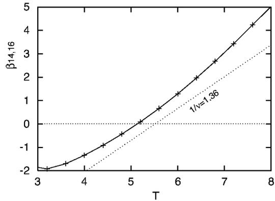
FIG . 3: We plotted the beta function,  $\beta_{1.4,1.6}(T)$  (10), for the same parameters as Fig. 2. From the slope at the transition point, we estimate the correlation-length critical exponent as  $\nu = 1.36$ .
