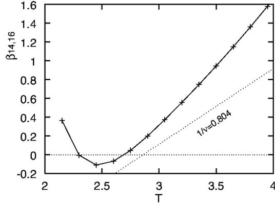
FIG .4: The beta function,  $\beta_{14;16}(T)$  (10), is plotted for  $j = 0:9$  and  $d_{\text{eff}} = 2.07$ . We notice that for  $d_{\text{eff}} = 2$ , the beta function gets curved, indicating that a nonstandard (essentially singular) criticality emerges. From the slope at the transition point, we estimate the correlation-length critical exponent as  $1/\nu = 0.804$ .
