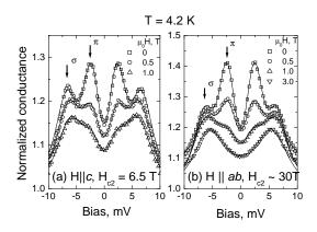
Fig 2. Representative experimental data at 4.2 K and corresponding best fits to Eq 2: (a) field parallel to the c axis; (b) field parallel to the ab plane.
