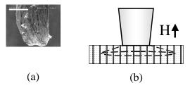
Fig 1. (a) Scanning electron microscopy image of the gold tip after the point-contact measurements. The scale bar corresponds to 50 microns. The size of the deformed tip apex is indicative of the contact dimensions. (b) Schematic representation of the contact probing a large number of Abrikosov vortices (vertical lines) with the current injected into a large solid angle (dashed lines).
