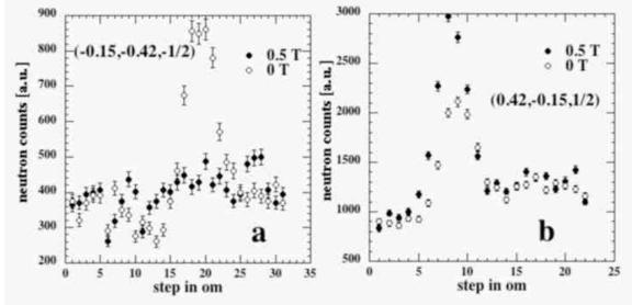
Fig. 4. The TriCS  $\omega$ -scans of the (-0.15,-0.42,-1/2) (a) and (0.42,-0.15,1/2) (b) magnetic reflections ( $\lambda$ =2.4 Å) at H=0 T and H=0.5 T along *a*.
