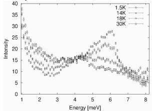
Fig. 6. Inelastic powder neutron scattering of Cu<sub>2</sub>Te<sub>2</sub>O<sub>5</sub>Cl<sub>2</sub> integrated between 0.8 Å<sup>-1</sup> and 3.3 Å<sup>-1</sup> for four temperatures between 2 K and 30 K. With incident energy  $E_i=10.4$  meV inelastic focusing was adjusted to provide optimal resolution at 5 meV of 0.45 meV (full-width-half-maximum). For single crystal neutron spectroscopy a single crystal was aligned with (3,1,0) and (0,0,1) in the horizontal scattering plane, such that
