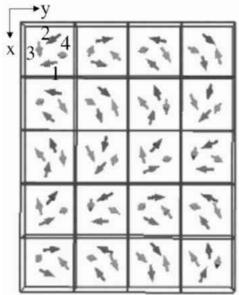
Fig. 5. The xy-projection of the  $Cu_2Te_2O_5Cl_2$  magnetic structure with the spin tetrahedra at the z=0 layer.
