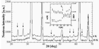
Fig. 2. The 18 K and 4 K DMC NPD patterns of Cu<sub>2</sub>Te<sub>2</sub>O<sub>5</sub>Cl<sub>2</sub> ( $\lambda$ =4.2 Å), arrows point to magnetic reflections. Inset: temperature evolution of the lattice constants from HRPT NPD data ( $\lambda$ =1.889 Å).
