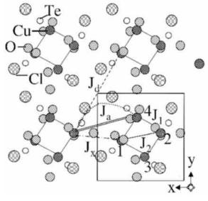
Fig. 1. The xy-projection of the  $Cu_2Te_2O_5Cl_2$  crystal structure (z=-1/2  $\div$ 1/2) with the J<sub>1</sub>, J<sub>2</sub> and possible intertetrahedral exchange paths [10]. The double-line segment is normal to the incommensurate component of the wave vector **k'** [8].
