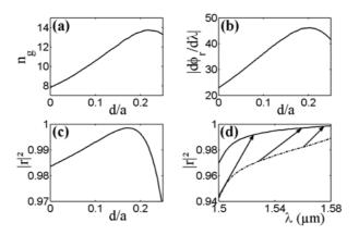
(a), (b) and (c) Effect of the holes shift on the main physical parameters involved in Eq. (2) for N = 3. (d)  $|r(\lambda)|^2$  for two mirrors with d = 0 (dashed-dotted curve) and d = 0.18a (solid curve). The arrows indicate the reflectivity change for the three cavities. From left to right, N = 1, 2 and 3.
