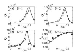
Comparison between experimental data (squares), calculation data (circles) and FP model predictions (solid curves). (a), (b) and (c) Q-enhancement for N = 1, 2 and 3, respectively. In (a), the FP model predictions do not show up for  $d \le 0.1a$ . For small *d*'s, the resonance wavelength is beneath 1.5 µm and the Bloch mode of the single-line-defect PC waveguide leaks in the air clads. (d) Resonance wavelength red-shift for N = 3.
