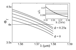
The total-phase delay  $\Phi_{\rm T}(\lambda)$  has been represented for d/a = 0, 0.05, 0.1, 0.15 and 0.25 and for N = 3. The phase-matching occurs for  $\Phi_{\rm T}(\lambda_0) = 4\pi$  (dashed horizontal line). Inset: dispersion diagram of the fundamental Bloch mode (solid curve). The dashed lines correspond to the resonance wavelengths for the above-mentioned values of *d*. From top to bottom, *d* increases.
