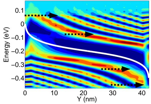
Fig. 9. Local density of states in the lowest non crossing subband of a (240,0) nanotube under a bias of 0.4 V as a function of position and energy. Brighter color shows higher DOS. Also shown is the potential profile. The arrows correspond to four contributions to a current due to the non crossing subband in Fig.10
