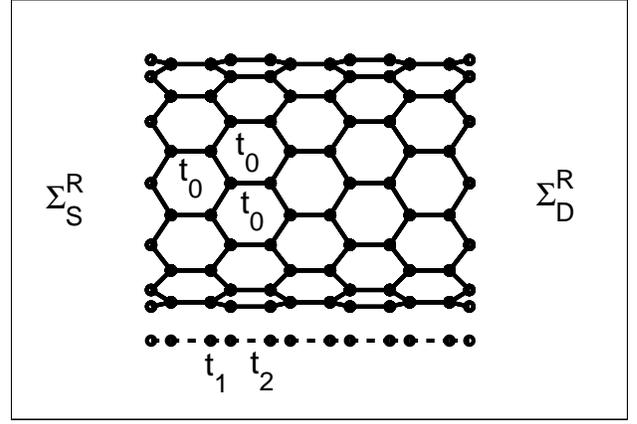
Fig. 1. Zigzag carbon nanotube and the corresponding 1D chain. The hopping parameter between nearest neighbors in the nanotube is  $t_o$ . The 1-D chain has two sites per unit cell with on-site potential  $U_o$  and hopping parameters  $t_1 = 2t_o \cos(\frac{\alpha}{2})$  and  $t_2 = t_o$
