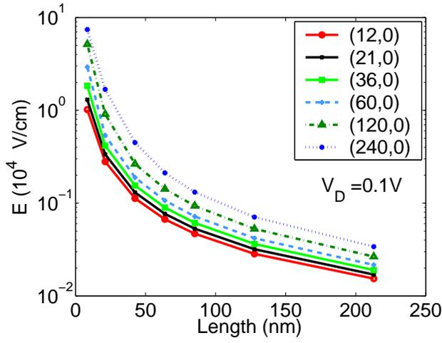
Fig. 5. This plot shows the electric field at the mid point versus nanotube length for various nanotube diameters at an applied bias of 100 mV. The electric field decreases approximately as  $1/L^{1.25-1.75}$ .
