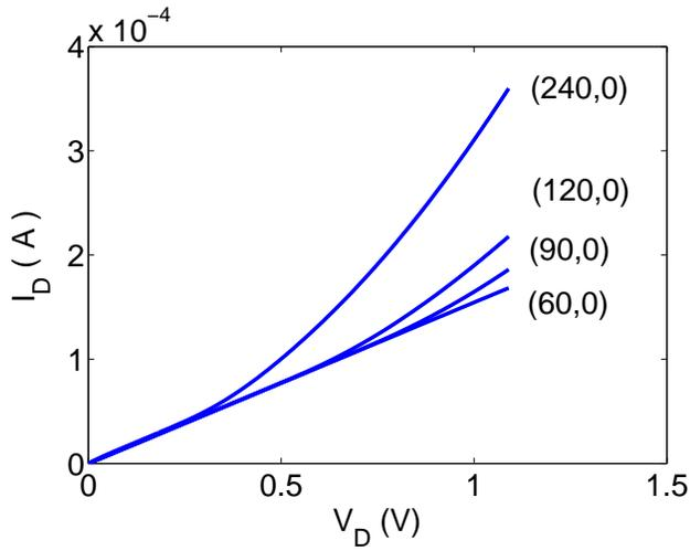
Fig. 7. The current-voltage characteristics of large diameter nanotubes in the ballistic limit. The current shows faster than linear increase with bias due to the contribution of non crossing subbands.
