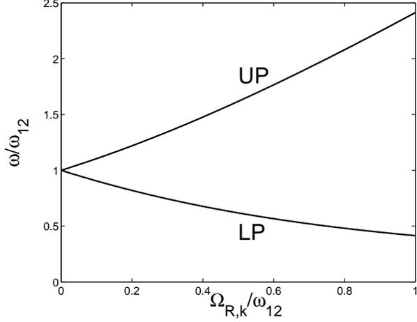
FIG. 3: Normalized polariton frequencies  $\omega_{LP,k}/\omega_{12}$  and  $\omega_{UP,k}/\omega_{12}$  as a function of  $\Omega_{R,k}/\omega_{12}$  for  $D_k = \Omega_{R,k}^2/\omega_{12}$ . The calculation has been performed with  $\omega_{cav,k} = \omega_{12}$ . Note that for a given microcavity system,  $\Omega_{R,k}/\omega_{12}$  can be tuned *in-situ* by an electrostatic bias, which is able to change the density of the two-dimensional electron gas.
