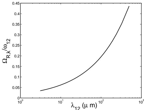
FIG. 2: Coupling ratio  $\Omega_{R,k}/\omega_{12}$  as a function of the intersubband emission wavelength  $\lambda_{12}$  ( $\mu\text{m}$ ). Parameters:  $f_{12} = 12.9$  (GaAs quantum well), cavity spacer refraction index  $\sqrt{\epsilon_{\infty}} = 3$ ,  $n_{QW}^{\text{eff}} = 50$ ,  $N_{2DEG} = 5 \times 10^{11} \text{ cm}^{-2}$  and  $\theta = 60^\circ$ . The Fabry-Perot resonator is a  $\lambda/2$ -microcavity. Results obtained from the analytical expressions in Eqs. (14) and (15).
