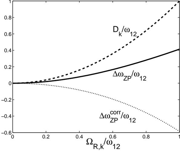
FIG. 5: Solid line: normalized differential zero-point energy (per mode)  $\Delta\omega_{ZP}(k)/\omega_{12}$  as a function of  $\Omega_{R,k}/\omega_{12}$ . Dashed line:  $D_k/\omega_{12}$ . Dotted line: normalized correlation contribution  $\Delta\omega_{ZP}^{corr}(k)/\omega_{12}$ . The calculation has been performed with  $\omega_{cav,k} = \omega_{12}$ .
