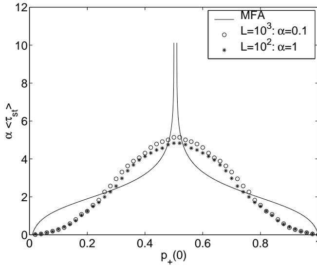
Figure 4: Mean relaxation times (divided by  $\alpha$ , to present results for  $L = 10^2$  and  $L = 10^3$  on the same plot) from the initial state, containing randomly distributed  $p_+ = (m_0 + 1)/2$  up-spins, to the ferromagnetic steady state. Obviously the mean field results are completely different from the simulation results. Moreover, comparison of the results for  $L = 10^2$  and  $L = 10^3$  clearly shows that no phase transition is present on the chain.
