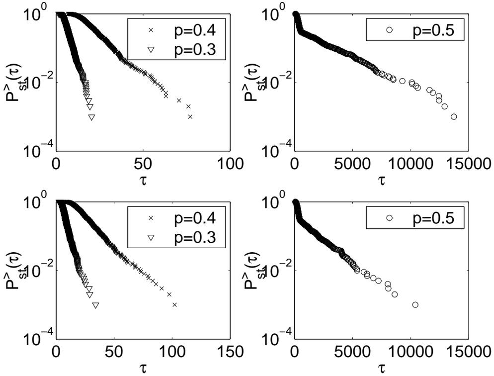
Figure 8: Probabilities of reaching the steady state in time larger than  $\tau$  on the square lattice for several values of the initial fraction of up-spins  $p$  for Stauffer (top) and Galam (bottom) generalizations of SM. The distribution of waiting times has an exponential tail with the exponent dependent on  $p$ . For both dynamics this dependence is identical. Critical slowing down is observed for  $p = 0.5$  (right panels).
