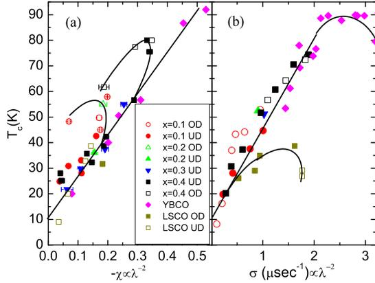
FIG. 10: (Color online) (a)  $T_c$  vs  $-\chi\sigma\lambda^{-2}$  at  $T = 1.6$  K for various samples of CLBLCO, YBCO and LSCO. (b)  $T_c$  vs the muon depolarization rate  $\sigma$  at  $T = 1.8$  K for the same CLBLCO samples. Data for YBCO and LSCO are from Ref. [14]
