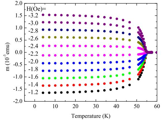
FIG. 4: (Color online) Field cooled magnetization vs temperature in a variety of fields, in the small field limit where  $H_0 = d^2$  and  $d$  is typical grain size.
