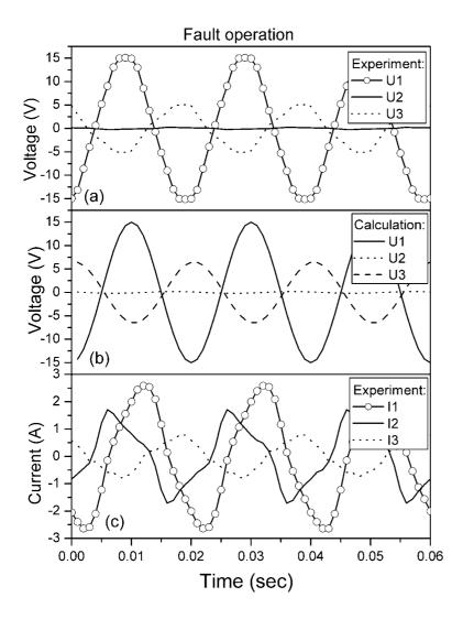
Fig. 3. Fault (HTS switch is in the normal state above the critical temperature of S-N transition): (a) – experimental waveforms of voltages; (b) – calculated waveforms of voltages at  $R_3 = 10$  Ohm,  $R_4 = 100$  Ohm; (c) experimental waveforms of currents.  $U_1$ ,  $I_1$  - voltage and current in the primary coil;  $U_2$ ,  $I_2$  – the main secondary coil;  $U_3$ ,  $I_3$  – the standby secondary coil.
