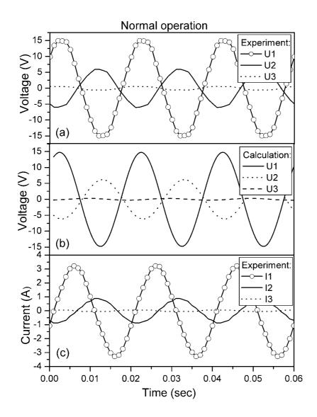
Fig. 2. Normal operating conditions (HTS switch is in the superconducting state): (a) – experimental waveforms of voltages; (b) – calculated waveforms of voltages at  $R_2 = R_3 = 10$  Ohm,  $R_4 = 0.006$  Ohm; (c) experimental waveforms of currents.  $U_1$ ,  $I_1$  - voltage and current in the primary coil;  $U_2$ ,  $I_2$  – the main secondary coil;  $U_3$ ,  $I_3$  – the standby secondary coil.
