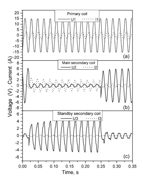
Fig. 4. Transient processes at a fault: (a) primary voltage  $U_1$  and current  $I_1$  (voltage and current are practically unchanged at a fault at 0.02 sec and at a fault clearing at 0.25 sec); (b) voltage  $U_2$  at the terminals of the main secondary coil  $W_2$ - $W_2$ ' and current  $I_2$  in the main line; (c) voltage  $U_3$  and current  $I_3$  in the standby line.
