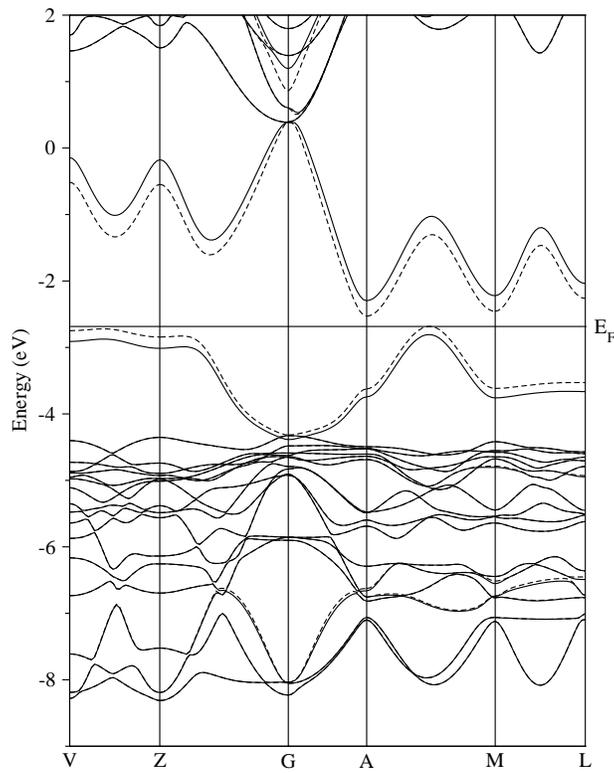
FIG. 6: BaBiO<sub>3</sub> band structure. Dashed lines shows LDA results and solid lines correspond to GTS calculations
