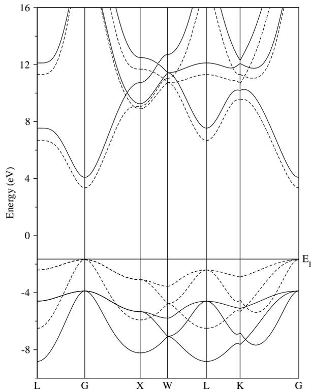
FIG. 2: MgO band structure. Dashed lines shows LDA results and solid lines correspond to GTS calculations
