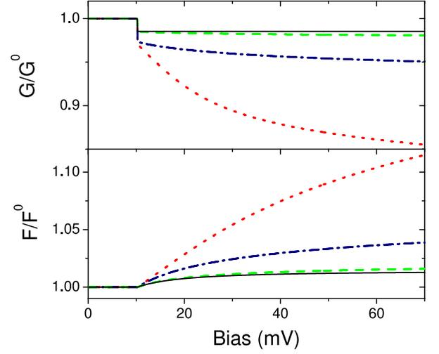
FIG. 2: Top panel: ratio of the total conductance  $G$  of an atomic gold point contact and its value in the absence of inelastic effects  $G^0$  as a function of bias for different values of thermal current coefficient (see text):  $A_{\text{th}} = 10^{19}$  (dot),  $10^{17}$  (dot-dashed),  $10^{15}$  (dashed), and 1 (solid)  $\text{dyn} = (\text{eK}^4)$ . Bottom panel: corresponding Fano factor ratio.
