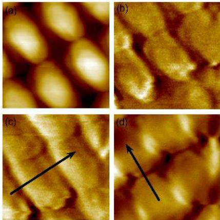
FIG. 2:  $1\ \mu\text{m} \times 1\ \mu\text{m}$  simultaneous topographic (a) and MFM (b) images of an array of elliptical permalloy particles at 4.2 K, with magnetic field  $H = 0$ . (c), (d) MFM images of the same sample at 4.2 K with an applied field of 2.5 kG. The magnetic field was applied in the direction shown by the arrows in the figures.
