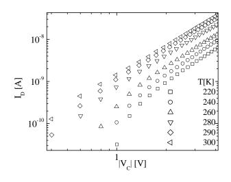
FIG. 8:  $I_D - V_C$  for devices with Cu electrodes ( $W = 400 \,\mu$  m) at  $V_G = -60$  V over a representative temperature range.
