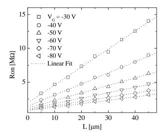
FIG. 2:  $R_{on}$  as a function of L at 300 K for a series of Au-P3HT OFETs with channel width of 200  $\mu$  m.
