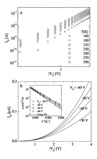
FIG. 7: Plots of extracted  $I_D - V_C$  data from a set of Cr electrode devices at (a) fixed  $V_G = -60$  V and several temperatures and (b) T = 210 K and several gate voltages. Inset in (b): Log-linear plot of  $\mu$  vs.  $T^{-1}$  for several gate voltages. The linear fit to the data indicates that the transport of carriers is dictated by simple hopping of carriers between localized states.
