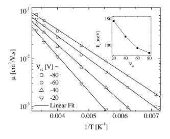
FIG. 4: Temperature dependence of the extracted channel mobility as a function of inverse temperature for a set of devices with Au source and drain electrodes at several gate voltages. Inset: Activation energies of the mobility as a function of the gate voltage
