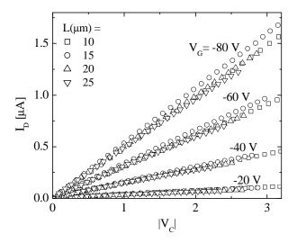
FIG. 3: Contact current voltage characteristics for the Au sample described in Fig. 2 at T = 250 K. At any given  $V_G$ , the data for different channel lengths is collapsed onto one, using an appropriate value for  $\mu$ . Therefore, the  $I_D - V_C$  data is unique for any  $V_G$  and T.
