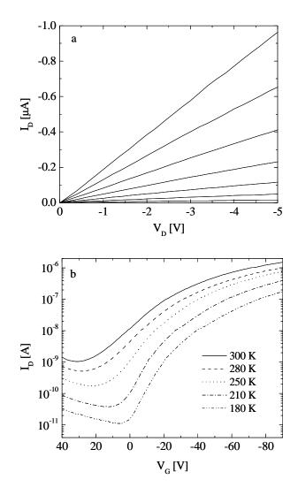
FIG. 1: (a) Transport characteristics of a P3HT OFET with Au source and drain electrodes, with  $L = 15 \,\mu$  m ,  $W = 200 \,\mu$  m at 300 K. The  $V_G$  s from top to bottom are -70, -60, -50, -40, -30, -20, -10 V. (b) Transfer characteristics of the same device for several temperatures at  $V_D = -3$  V.
