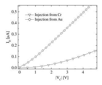
FIG. 6: Extracted  $I_D - V_C$  for a series of devices of width  $200 \,\mu$  m with alternating Cr and Au electrodes at 240 K and  $V_G = -80$  V. Upper curve shows injection of holes from Au, while the lower curve shows injection from Cr. Injection from Au is more linear and allows higher currents at lower voltages.
