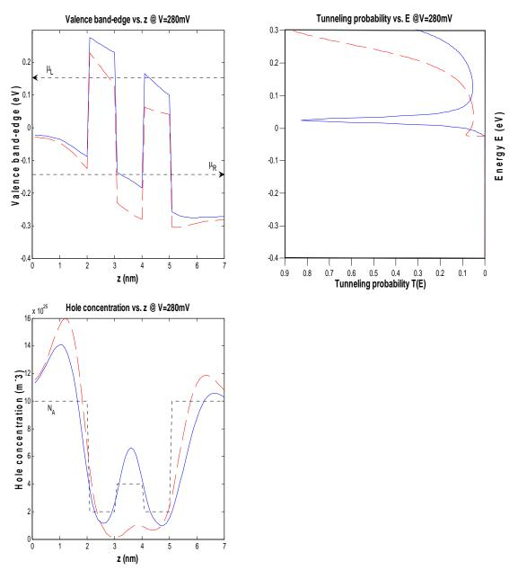
FIG. 2. (Color Online) Paramagnetic state: V=280mV; solid (blue) lines denote the forward path (increasing voltage) and broken (red) lines denote reverse path (decreasing voltage). The former is the current-carrying state with large charge accumulation. In dotted lines:  $\mu_L$ ,  $\mu_R$  are the chemical potentials in the left and right leads, N<sub>A</sub> is the acceptor doping profile.
