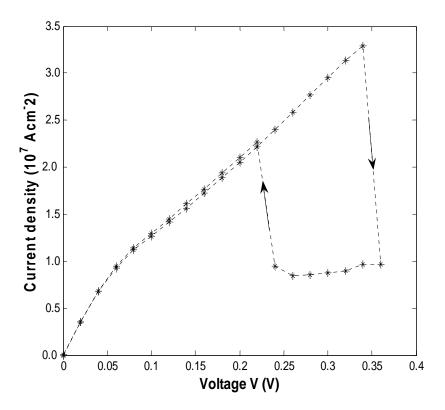
FIG. 1. Hysteretic current voltage (I-V) characteristics of the ferromagnetic well resonant tunneling diode.
