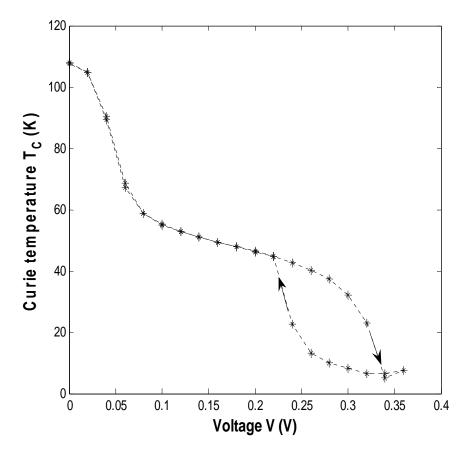
FIG. 3. Hysteretic Curie temperature vs. voltage ( $T_C$ -V) characteristics of the ferromagnetic well resonant tunneling diode.
