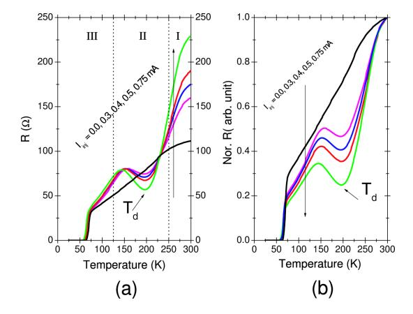
Fig. 2 Temperature-dependent in-plane resistance R (T) for the YBCO layer in Fig (a) for different SPQ currents (a). Note, that an enhancement of the SPQ current causes an increase of the resistance at room temperature, but a drop of the resistance is found around the temperature of the order of 25%. Additionally, a shift from ~63K to ~54K is found in the transition temperature  $T_c$ . (b) Normalized temperature-dependence of the in-plane resistance.
