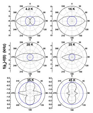
FIG. 3 (color). Polar plot of angular dependence of frequency shifts for an in-plane 5 kOe field. The field angle is measured relative to [110]. Note the change of scale on the axes. The  $\Delta f=0$  reference line is shown in blue.
