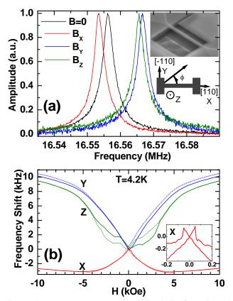
FIG. 1 (color). (a) Frequency response of the device for various 10 kOe field directions (Z is out of the plane). Amplitude is normalized for clarity. INSET. SEM image of the suspended (Ga,Mn)As beam and Au side gate with the axis directions. (b) Frequency shift dependence on field magnitude and direction. Dotted curves are for reversed field sweep direction. INSET. Expanded view of shifts in a field along X, showing domain wall-induced transitions.
