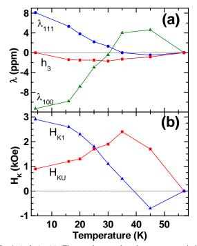
FIG. 4 (color). (a) First and second order magnetostriction constants of  $Ga_{0.948}Mn_{0.052}As$ . (b) First order cubic and in-plane uniaxial anisotropy fields.
