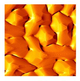
**Figure 2:** Scanning tunneling microscope image  $(345 \times 345 \text{ nm})$  of the surface of a crystalline platinum film after deposition of 93 atomic layers at a temperature of 440 K. New islands nucleate on top of the pyramidal mounds and grow until they reach the size of the underlying triangular terrace. Top terraces of different sizes represent different stages in this growth process.
