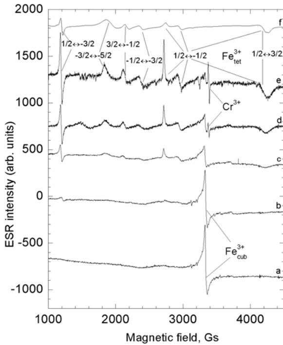
**Figure 5.** ESR spectra at  $T = 20^\circ\text{C}$  in nanopowder  $\text{BaTiO}_3$ : 0.01 % Fe samples annealed at different temperatures: a –  $900^\circ\text{C}$ , b –  $1000^\circ\text{C}$ , c –  $1100^\circ\text{C}$ , d –  $1200^\circ\text{C}$ , e –  $1350^\circ\text{C}$ ; f – calculated spectrum in tetragonal phase of  $\text{BaTiO}_3$ .
