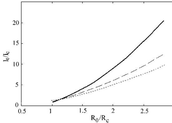
**Figure 4.** Size dependence of ratio of the integral intensities of axial and cubic absorption lines for different parameters of distribution function  $R_0/\sigma$ : 2.4 (dotted line); 2.8 (dashed line); 3.5 (solid line).
