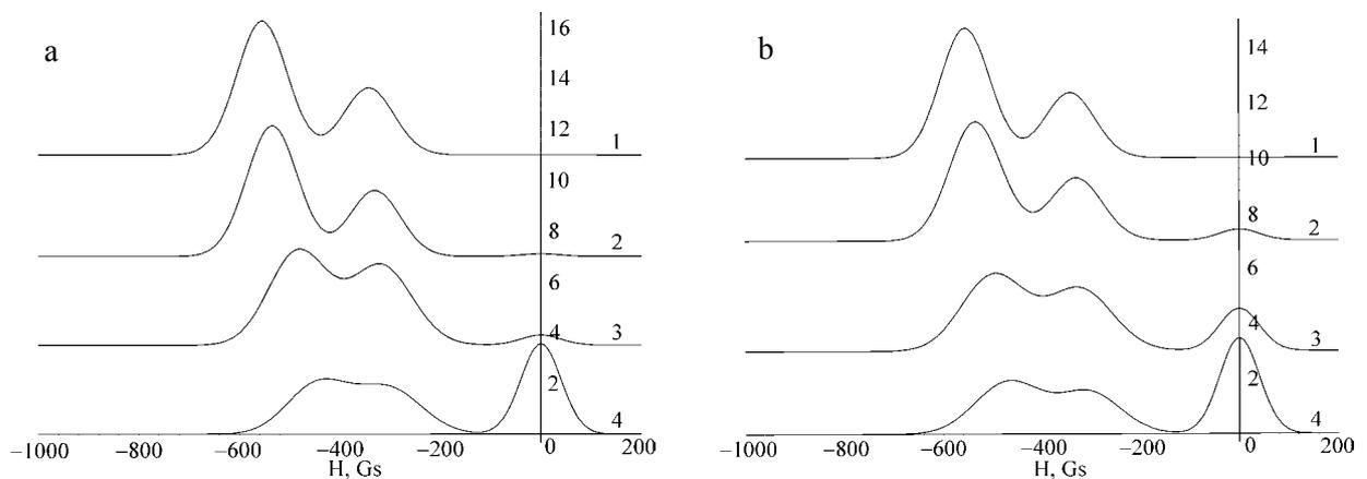
**Figure 1.** Calculated ESR absorption spectra of paramagnetic probe with inversion center for several nanopowder ferroelectrics with  $I^{\text{st}}$  order phase transition. The parameters of size distribution function are the following:  $R_0/R_c = 5$  (1), 3 (2), 2.1 (3), 1.2 (4);  $\sigma/R_c = 0.7$  (a), 1.4 (b).
