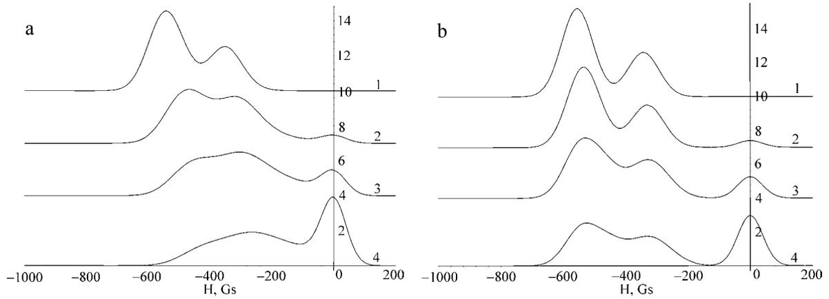
**Figure 2.** Calculated ESR absorption spectra of paramagnetic probe with (a) and without (b) inversion center for several nanopowder ferroelectrics with II<sup>st</sup> order phase transition. The parameters of distribution function are the same as in Fig. 1,b.
