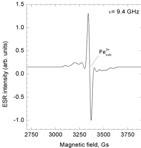
**Figure 6.** Calculated ESR spectrum for  $\text{Fe}^{3+}$  ions in cubic phase of  $\text{BaTiO}_3$  powders.
