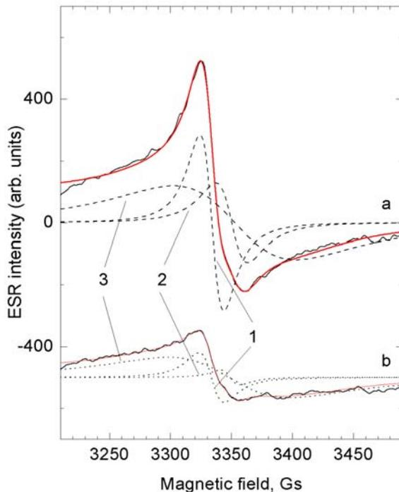
**Figure 8.** ESR spectra (solid lines) in nanopowders BaTiO<sub>3</sub> annealed at 900°C (a), 1100°C (b). Dash lines – the results of the spectrum deconvolution correspondingly: 1 – core, 2 – shell, 3 – the residuals of tetragonal lines.
