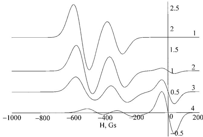
**Figure 7.** Calculated ESR spectra in the form of derivatives for powder samples with the size distribution function in the form of one Gaussian (for curves 1 and 2) and of two Gaussians (for curves 3 and 4) with parameters  $R_0/R_c = 5$  (1), 3 (2);  $R_{01}/R_c = 2.1$  and  $R_{02}/R_c = 4.5$  (3);  $R_{01}/R_c = 0.9$  and  $R_{02}/R_c = 2.8$  (4).
