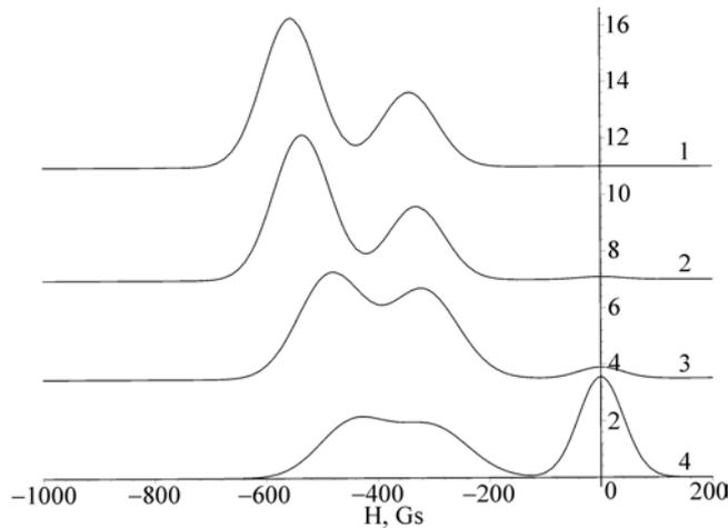
**Figure 3.** Calculated ESR absorption spectra of paramagnetic probe with inversion center for nanopowder ferroelectrics with I<sup>st</sup> order phase transition and size distribution function in the form of one Gaussian (for curves 1 and 2) and of two Gaussians (for curves 3 and 4).
