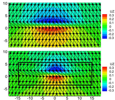
FIG. 2: Dislocation core structures obtained from the EAM-based QC (top) and the present QCDFD method (bottom). The black circles are atoms. The contours correspond to out-of-plane ( $z$ ) displacement in Å. The contours clearly indicate the splitting of the dislocation. The atoms within the black box in the bottom panel are DFT atoms. The finite element mesh serves no other purpose in this nonlocal atomistic region other than as a guide to the eye to help visualize deformation.
