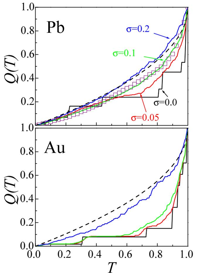
FIG. 4: (Color on-line). Effect of atomic disorder in the calculated distributions  $Q(T)$  for Pb and Au. The curves correspond to different values of the disorder parameter  $\sigma$  described in text: 0 (black line), 0.05 (red), 0.1 (green) and 0.2 (blue). The symbols correspond to an average of the experimental results from 10 to  $15G_0$ . The dashed line corresponds to the universal diffusive distribution.
