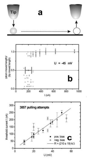
**Fig. 4** Lateral manipulation (LM). (a) A schematic drawing shows the tip action during LM. (b) The probability to move an atom vs. tunneling current at -45 mV. (c) At the small bias range, the threshold current linearly varies with the bias.  $R_t$  can be determined from the slope of this curve.
