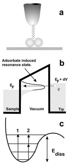
Fig. 10 IET manipulation. (a) A schematic drawing shows an IET dissociation. (b) Inelastic tunneling electrons are injected to the molecule through an adsorbate-induced resonance state. (c) Single and multiple excitation processes in case of IET induced bond breaking.
