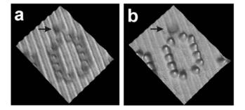
**Fig. 9** Imaging with a CO-tip. (a) The CO molecules that form '0' on a Cu(211) surface appear as depressions when imaged with a normal tip. (b) The CO molecules appear as protrusions when imaged with a CO-tip. An unknown adsorbate (shown with arrow) is still remains as a depression in both images, thus chemical contrast is achieved [Courtesy of J. Repp, IBM Zurich].
