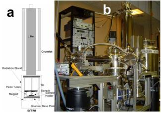
Fig. 1. Low-temperature STM for single atom/molecule manipulation. (a) A schematic drawing of STM scanner set-up. (b) An image showing a custom-built UHV-LT-STM system at the author's lab.
