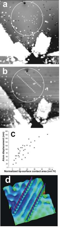
Fig. 2 STM images of tip indentations. (a) An STM image of Ag(111) surface after a tip-crash. (b) An STM image acquired after the second tip-crash, which produces a sharper triangular shape hole. [Imaging parameters:  $V_t = 0.29 V$ ,  $I_t = 1.7 nA$ , scan area = 120 x 120 nm<sup>2</sup>].
