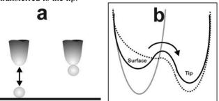
**Fig. 8.** Vertical manipulation (VM). (a) A schematic drawing shows the process. (b) The double-potential well model. The black (solid), dash and gray curves represent the shape of potentials (the well shapes are working assumptions) at an image-height, under an electric field, and at the tip-atom/molecule contact, respectively.
