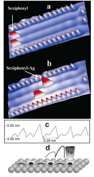
Fig. 12. Molecular shooting: (a) Two sexiphenyls (left) and two target atoms (right) are positioned along the standing wave track. A
