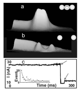
**Fig. 11.** Iodine abstraction. (a) An adsorbed p-diiodobenzene ( $C_6H_4I_2$ ) molecule at Cu(111) a screw dislocation. (b) After breaking the two C-I bonds of the molecule using IET process, the two iodine atoms remain adsorbed. (c) The changes in the current (shown with arrows) are due to bond-breaking events. Inset shows the C-I bond dissociation probability collected from 70 dissociations.
