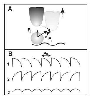
**Fig. 5.** (a) The drawing demonstrates the vertical and parallel force components involved in LM. (b) STM tip-height manipulation curves correspond to (1) pulling, (2) pushing, and (c) sliding modes.
