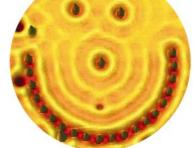
**Fig. 7.** OU logo writing sequence using individual silver atoms on a Ag(111) surface at 6 K (upper) and a three dimensional representation (middle) (42 nm x 26 nm area, 51 silver atoms are used). The "atomic smiley" image is written by using silver atoms on a Ag(111) surface at 5 K (32 nm diameter).
