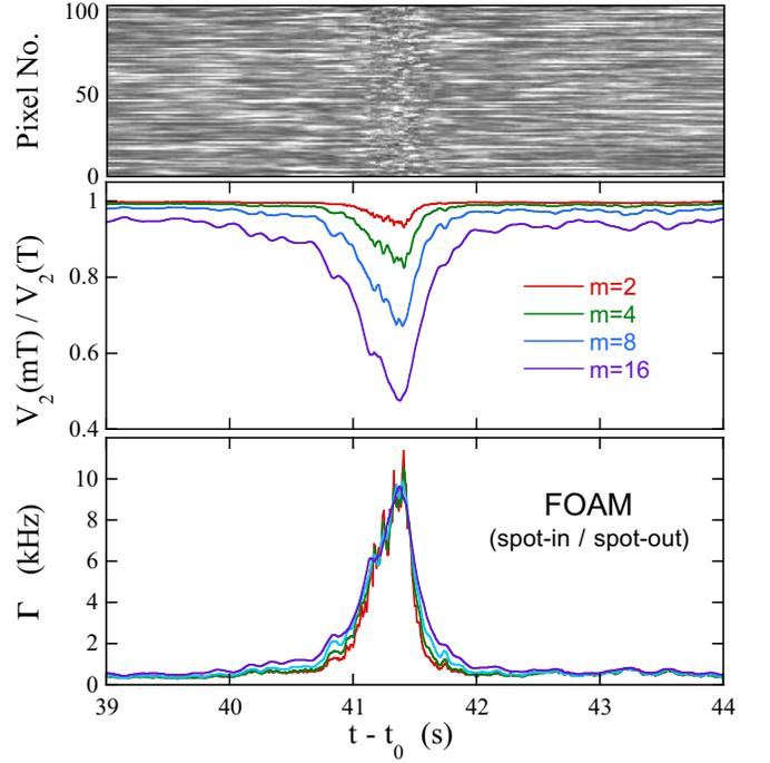
FIG. 10: Pixel grayscale levels, variance ratios, and Lorentzian linewidths as a function of age for a coarsening foam. The offset along the time axis is  $t_0 = 6$  hrs, the lapse between sample production and the beginning of data collection. Here the exposure duration is  $T = 10$  ms.
