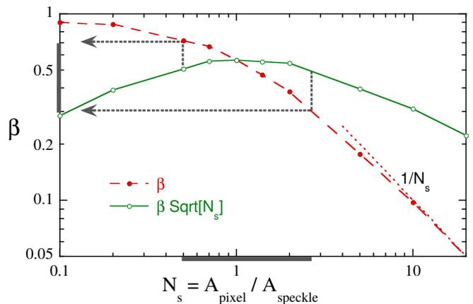
FIG. 7: The intercept or maximum speckle contrast,  $\beta = v_2(0) = \langle I^2 \rangle / \langle I \rangle^2 - 1$ , and the figure of merit  $\beta\sqrt{N_s}$  to be maximized in design of experiment, as a function of the number  $N_s$  of speckles per pixel. An experiment with polarized detection is within about ten percent of optimal if the intercept lies in the range  $0.3 < \beta < 0.7$ .
