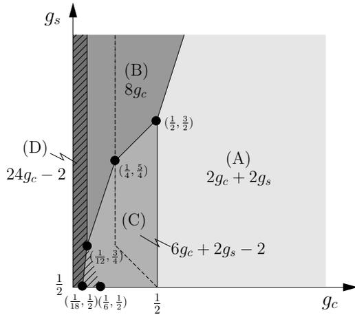
FIG. 3: Diagram for the leading power-law contributions to the rectification current,  $I_r \sim V^z$ , for voltages  $V \gtrsim V^*$ . The exponents  $z$  for the four different phases are given by the formulae in the figure (see also Table I). The zone boundaries indicate crossover regions. On the left of the dashed line  $V^* > 0$ , and on the right  $V^* = 0$  (see Eq. (11)). In the hatched area,  $z < 0$ , and the rectification current shows the behavior sketched in Fig. 2.
