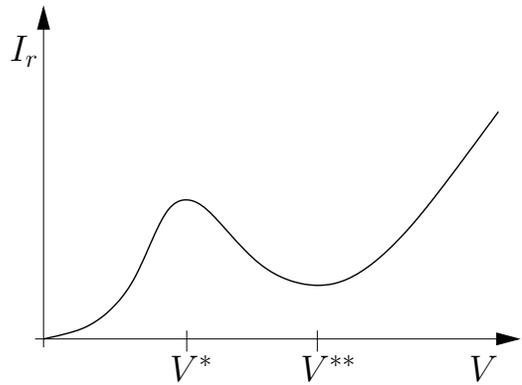
FIG. 2: Qualitative behavior of the rectification current,  $I_r(V) = [I(V) + I(-V)]/2$ , in the region, where the leading (third order) exponent is negative,  $z < 0$ . For voltages larger than  $V^*$ , the rectification current decreases until, at  $V^{**}$ , the leading second order term exceeds the third order amplitude, and leads to a further increase of the current.
