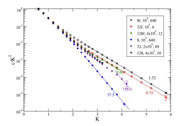
FIG. 3: 2D  $\pm J$  spin-glass reduced specific heat  $c/K^2$  vs. K. The legend specifies the lattice size L (f for free boundary conditions), Monte Carlo steps, and number of samples of random couplings. The straight lines are fit to  $c/K^2 \approx b \exp(-2K)$  or  $b \exp(-4K)$ , with b indicated on the lines. The errors at the largest K are mainly due to sample fluctuations.
