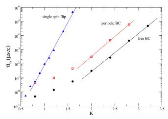
FIG. 2: Correlation times,  $\tau t_0$ , measured in actual CPU times for single-spin-flip, 1-step N-fold-way worm algorithm with periodic boundary condition and with a free boundary condition, for L=128. The slopes a of the straight line fits to  $\exp(aK)$  are 14.0, 6.5, and 6.2, respectively.
