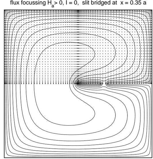
FIG. 9: The current stream lines in a thin superconductor square ( $|x| \leq a$ ,  $|y| \leq a$ ) with radial slit running at  $y = 0$  from  $x = 0$  to  $x = a$ , with a superconducting bridge at  $x = a_2 = 0.35a$ . Shown is the flux-focussing case  $H_a > 0$ ,  $I = 0$ , i.e., no current crosses the bridge.  $\Lambda/a = 0.01$ . The dots mark the numerical grid of  $80 \times 80$  points used for this plot.
