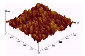
Fig. 1: AFM image of a V<sub>2</sub>O<sub>3</sub> thin film deposited on LiNbO<sub>3</sub>.
