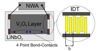
Fig. 3: Schematic view of a surface acoustic transmission line: A  $V_2O_3$  film on top of LiNbO<sub>3</sub> together with an enlarged view of the IDT structure. Bond contacts serve for dc resistivity measurements.
