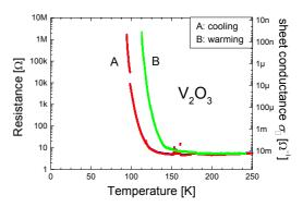
Fig. 4: Temperature dependence of the resistance and sheet conductance  $\sigma$ , respectively, of a V<sub>2</sub>O<sub>3</sub> film on LiNbO<sub>3</sub> substrate.
