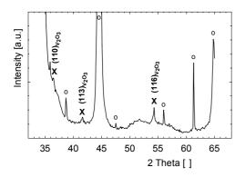
**Fig. 2:** XRD measurements of a  $V_2O_3$  thin film (d=370 nm) deposited on LiNbO<sub>3</sub>. X:  $V_2O_3$  peaks; o: Substrate and sample holder peaks.
