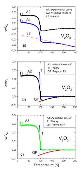
Fig. 7: Velocity shift vs. temperature for cooling down.
