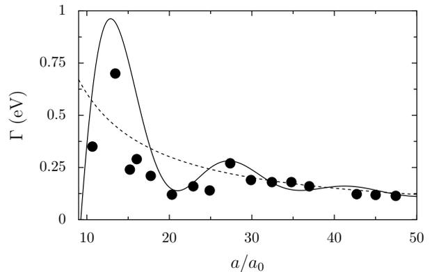
FIG. 2: Inverse lifetime of the first collective excitation in Na nanoparticles as a function of the radius  $a$  of the particle. The dashed line is the smooth part of the single plasmon linewidth, Eq. (1). The full line is the smooth part plus the oscillating contribution from Eq. (18) for a number of repetitions  $\tilde{r} = 1$ . This semiclassical result is compared to numerical TDLDA calculations (dots) for clusters with magic numbers of atoms between 20 and 1760.
