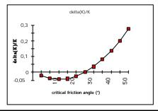
**Figure 1:** Comparison between the oedometric modulus  $k_{oedometric}$  as calculated from triaxial test result, i.e.  $k_{oedometric} = \sigma_3/\sigma_1 = [1+(8M+9)^{1/2}]/[4M+4]$ , and the experimental best fit of Jaky, i.e.  $k_{jaky} = 1$ -sin  $\phi$ , vs. the friction angle  $\phi$  of perfect plasticity. Fig. 1a: the two dependencies. Fig. 1b: their relative difference.
