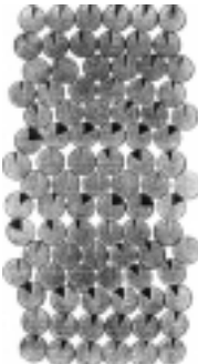
Figure 4: Calculation performed with Trubal 2d by Mahboudi & Cambou of the deformation of a square lattice of rods under uniaxial vertical compression.
