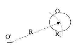
Indeed, to do so, one shall note first that tore-like flow lines are generated by inertia in any closed cell filled with liquid that is started rotating. So, let us consider a cylindrical finite closed cell of radius  $R_{\rm t}$ , centred on point O, on which a periodic motion is imposed; let us fill it up with liquid and sand and let us also assume that the periodic motion consists of a periodic rotation around a point O' which might be different from O . Let us note R the distance OO'.
