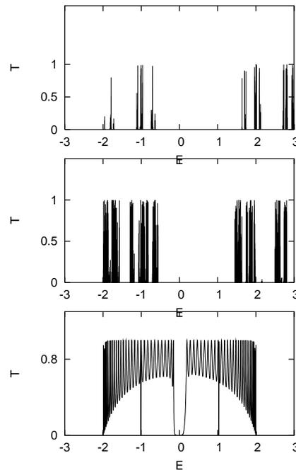
FIG. 3: The transmittivity ( $T$ ) against energy of a seventh generation 3-simplex fractal. The top figure corresponds to the isotropic case with  $t_x = t_y = T_x = T_y = 1$ . The middle and the bottom ones depict the situation with  $t_y = T_y = 0.9$  and  $t_y = T_y = 0.1$  respectively. The on-site potentials are kept constant at  $\epsilon_\alpha = \epsilon_\mu$  in each case. The lead parameters are,  $\epsilon_0 = 0$ , and  $t_0 = 2$ .
