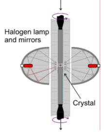
**Figure 8** Outline of the principles for a floating zone mirror furnace. The crystal is grown by moving sintered powder rods through an optically heated floating zone.
