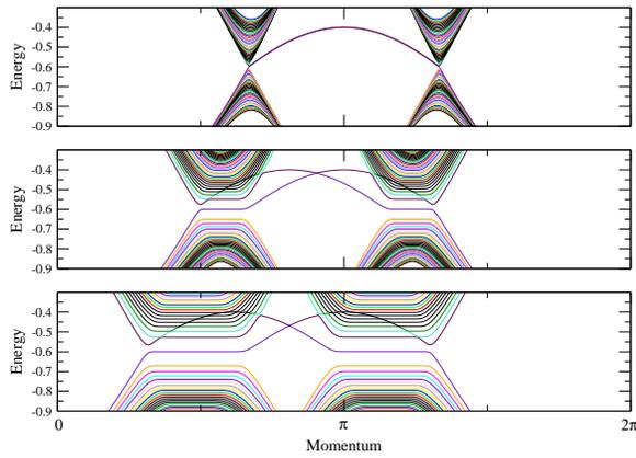
FIG. 2: Energy levels of a graphene ribbon of width 600 a with zig-zag edges as function of the momentum parallel to the edges. Energy in units of  $t$ , and  $t^0 = 0.2t$ . Momentum in units of  $1/(2 \cdot 3a)$ . Top: zero magnetic field; Centre: a magnetic flux per C atom of  $= 0.00025 \phi_0$ ; Bottom:  $= 0.0005 \phi_0$ .
