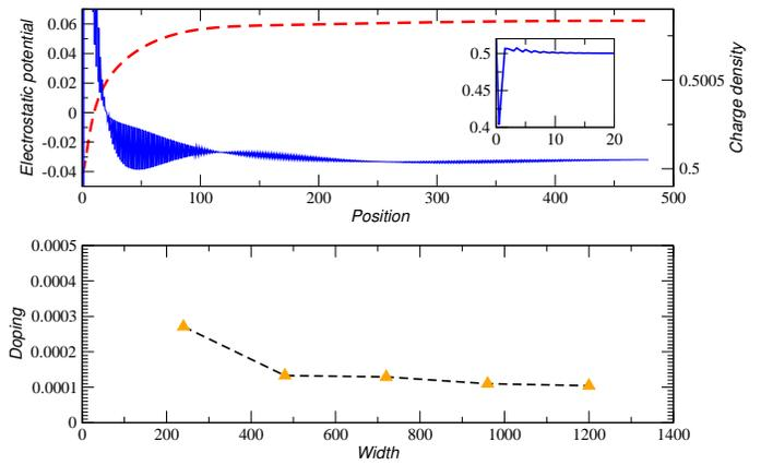
FIG. 1: Top: Electrostatic potential (dashed line) and electronic charge (continuous line) as a function of position along a long graphene ribbon terminating on a zig-zag edge. Energies are given in units  $t$ , and distances in units of  $a$ . We have used  $\tau^0 = 0.2t$ , and  $e^2/\epsilon_0 a = 0.5$ . The inset shows the details of the electronic density near the edge. Bottom: Total additional charge per C atom in extended states as function of the ribbon width,  $W$ .
