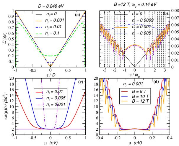
FIG. 3: (a): Density of states as function of vacancy concentration ( $D$  is a high energy cut-off); (b): As in (a), in the presence of an applied field. Dashed lines mark the positions of the Landau levels in the absence of disorder; (c) and (d):  $\pi\sigma(\mu)/2e^2$  as function of the Fermi energy  $\mu$ .  $t^0 = 0$  in all cases.
