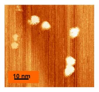
**Figure 2**: STM micrograph of Pd nanocrystals on HOPG substrate.
