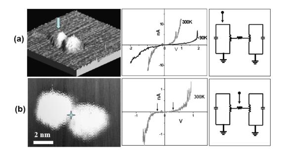
**Figure 4**: Tunneling microscopy and spectroscopy on a dimer of nanocrystals at 300 and 90 K. STM micrographs are shown on the left, I-V data in the middle and schematic circuits on the right side, a) an isometric view, the tip bias being applied to one of the nanocrystals is shown with an arrow, b) a top view with tip bias applied to the central region, as marked.
