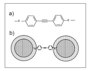
**Scheme 1**: (a) Dimercaptodiphenylacetylene (dmdpa) (b) A schematic showing a dimer of Pd nanocrystals linked by a dmdpa molecule.
