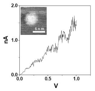
**Figure 3**: I-V data from an isolated Pd nanoparticle showing a coulomb staircase behavior. Inset shows the STM micrograph.
