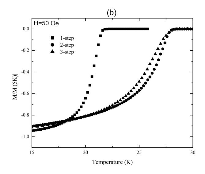
Fig. 7. (a) (002) and (110) x-ray peaks for nominal  $Mg(B_{0.8}C_{0.2})_2$  using  $B_4C$  as the boron and carbon source and reacted using 1, 2, and 3 step reaction processes. (b) Normalized magnetic transitions for these samples.
