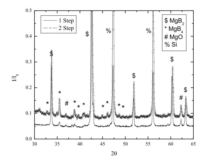
Fig. 3. Normalized powder x-ray pattern for a sample with  $x_n=0.05$  synthesized using a one step and a two step reaction. The two step sample clearly contains enhanced amounts of MgB<sub>4</sub>.
