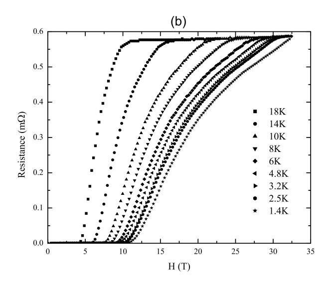
Fig. 8. (a) Resistance versus temperature and (b) resistance versus field for a sample with  $x_{i2}=0.069$ .
