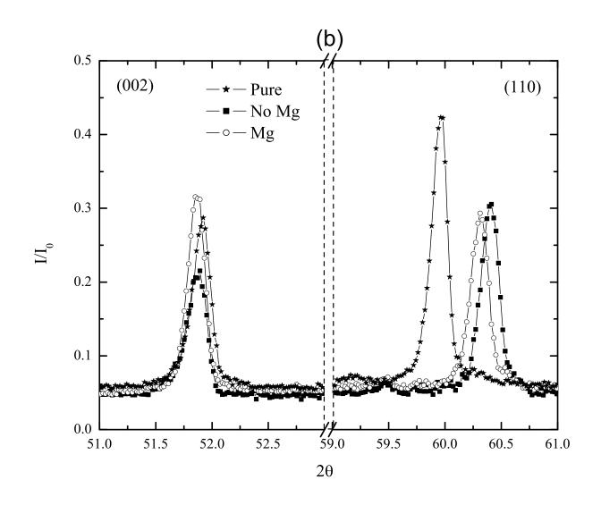
Fig. 4. (a) Normalized magnetization curves and (b) x-ray (002) and (110) peaks for a sample of  $x_n=0.05$  reacted using a two step process. If the second sintering step is performed without any excess Mg to compensate for potential losses, the resultant carbon content within the MgB<sub>2</sub> phase is increased.
