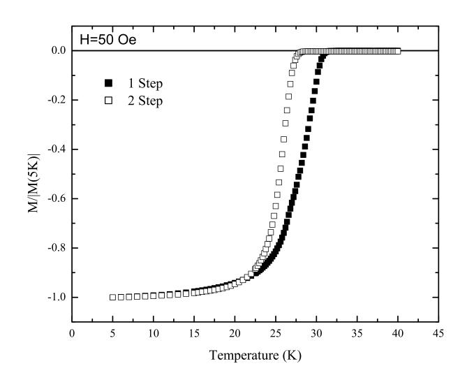
Fig. 2. Normalized magnetization curves for nominal  $Mg(B_{.95}C_{.05})_2$  samples. The second sintering step lowers  $T_c$ , consistent with the incorporation of a higher carbon concentration.
