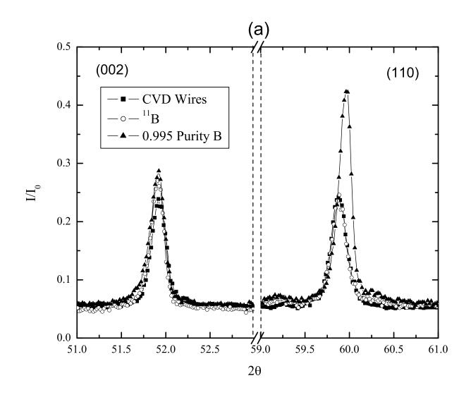
Fig. 11. Comparison of (002) and (110) x-ray diffraction peaks for pure MgB<sub>2</sub> made using different purity boron as the starting material. The 0.995 purity shows a shift in the (110) peak which presumably is not a result of inadvertent carbon doping.
