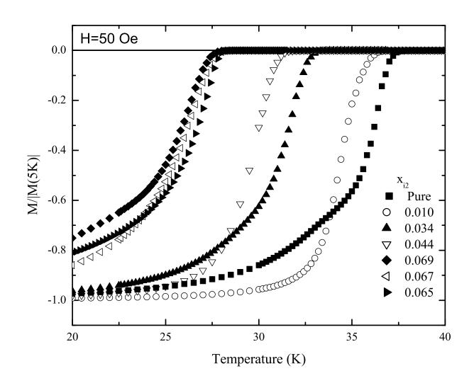
Fig. 6. Normalized magnetic transitions for the series of  $Mg(B_{1-x}C_x)_2$  with  $x_{i2}=0.01, 0.034, 0.044, 0.069, 0.067, 0.065$ , synthesized with 0.995 purity B and reacted using a two step process.
