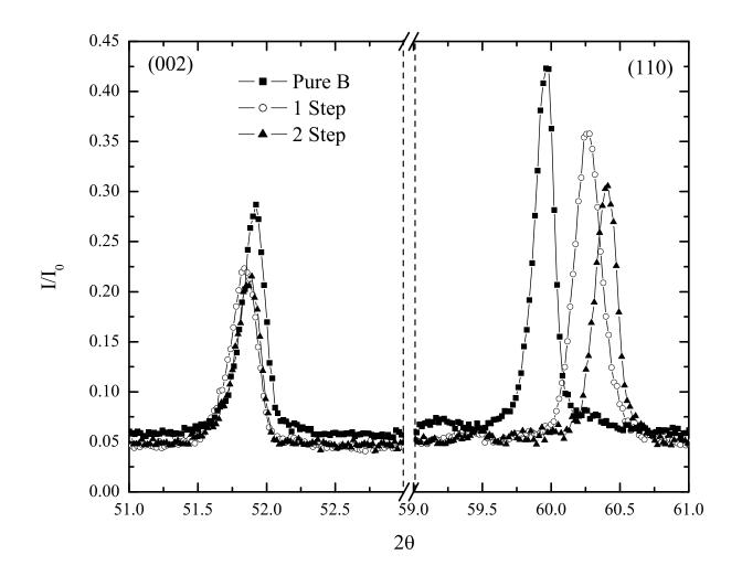
Fig. 1. Powder x-ray diffraction (002) and (110) peaks for pure and nominal  $Mg(B_{.95}C_{.05})_2$  samples made using the 0.995 purity boron as the starting material. The pure sample was reacted using two steps. For the carbon doped sample, the second sintering step shifts the (110) peak position to higher  $2\theta$  indicating the incorporation of a higher carbon concentration.
