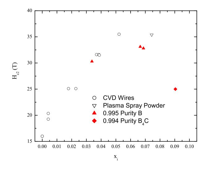
Fig. 12.  $H_{c2}(T=0)$  curves for the samples with different purity in the starting boron. CVD wires and plasma spray powders are from references [12] and [24] respectively.  $H_{c2}$  data on the highest doping level is from reference [25].
