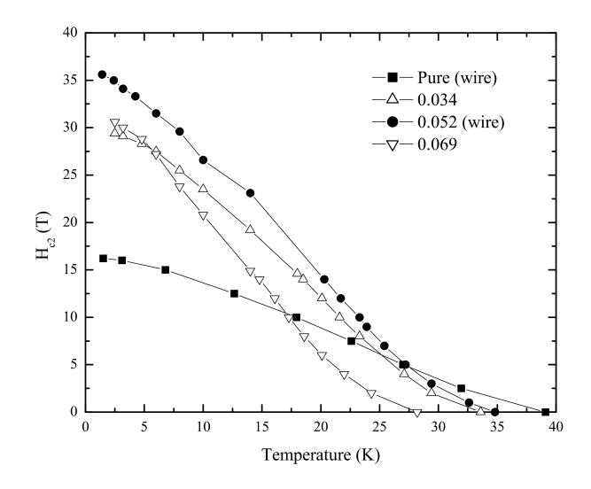
Fig. 9. Comparison of upper critical field curves for pellets with carbon doping levels of  $x_{i2}=0.034$  and 0.069 with wires containing  $x_i=0$  and 0.052. The  $x_i=0$  and 0.052 samples were made by reacting Mg vapor with boron filaments, see reference [7].
