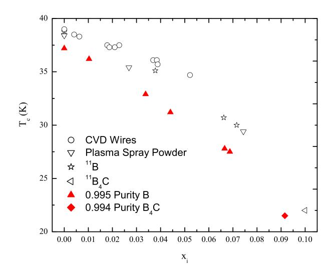
Fig. 10. Evolution of  $T_c$  as a function of  $x_i$ . CVD wires and powders are from references [12] and [24] respectively. Data on the sample prepared with isotopically enriched <sup>11</sup>B<sub>4</sub>C is from reference [20].
