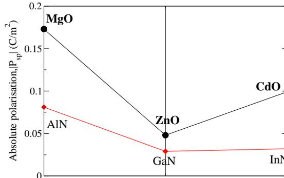
FIG. 2: Calculated absolute polarization values of the II-VI oxides ZnO, MgO and CdO (this work) and their III-V nitride analogues GaN, AlN and InN (from Ref. 15).
