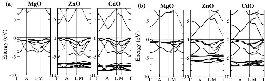
FIG. 1: Band structures of MgO, ZnO and CdO within (a) pseudo-SIC and (b) LDA approaches, at the calculated optimized LDA lattice parameters. Notice that the LDA severely underestimates the band gap, and results in a metallic ground state for CdO; this prevents the calculation of the polarization and piezoelectric coefficients.
