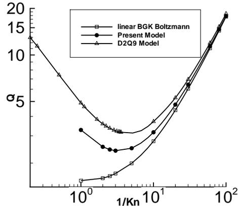
FIG. 1: Flow rate in the pressure driven Poiseuille flow as a function of inverse Knudsen number. Comparison of the present energy-conserving model with the isothermal lattice Boltzmann model *D2Q9* [13] and the continuous linearized Boltzmann-BGK model [14].
