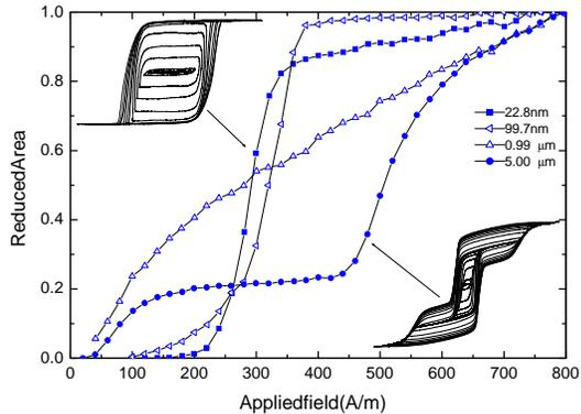
Fig. 1. Hysteresis loop area for Finemet thin films at different thicknesses. The area is divided by the value at  $H=800$  A/m for convenience. Examples of minor loop measurements are shown for the thinnest (22.8 nm) and the thickest (5  $\mu\text{m}$ ) sample.
