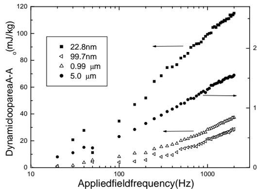
Fig. 2. Frequency dependence of the dynamic hysteresis area  $A - A_0$  obtained by fluxometric measurements. Data for the thickest sample are obtained considering only the inner loops not showing the double switching as in Fig. 1.
