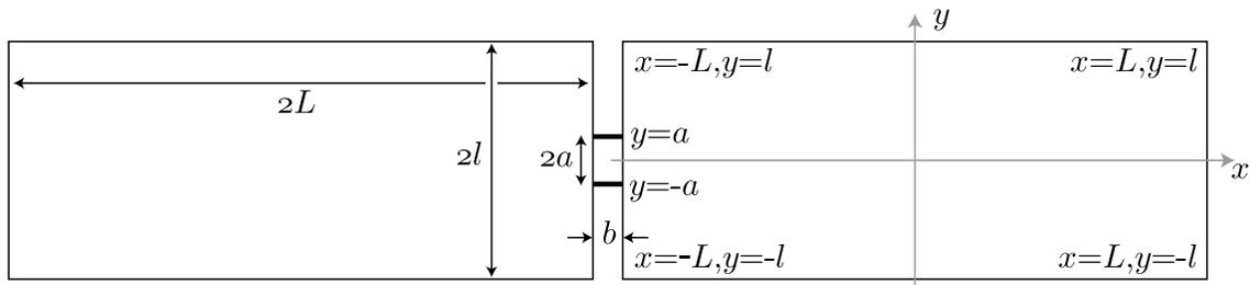
FIG. 2: Geometry of the two-wire device, showing the dimensions. The coordinate system used for the right lead (with the origin in the center of the lead) is also shown. The coordinates of the four corners of the right lead, as well as the coordinates of the points at which the two wires are connected to the right lead, are indicated. As shown, we always assume that the wires are attached near the center of the short edges of the leads.
