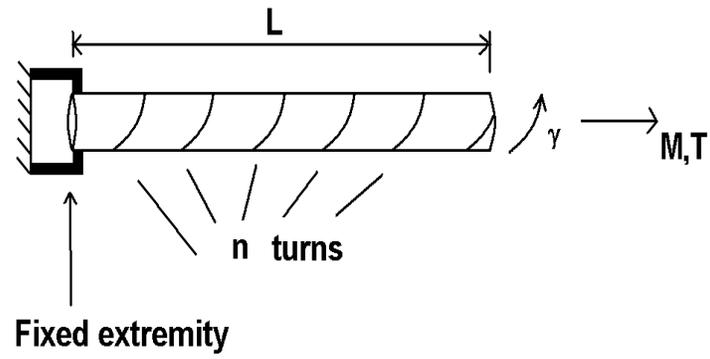
FIG . 1: Outline of the experimental setup to measure the elastic constants  $E$  and  $\nu$ . A torque  $M$  is applied along the axis of the rod, creating a twist density  $\gamma$ .  $T$  is the force of tension.
